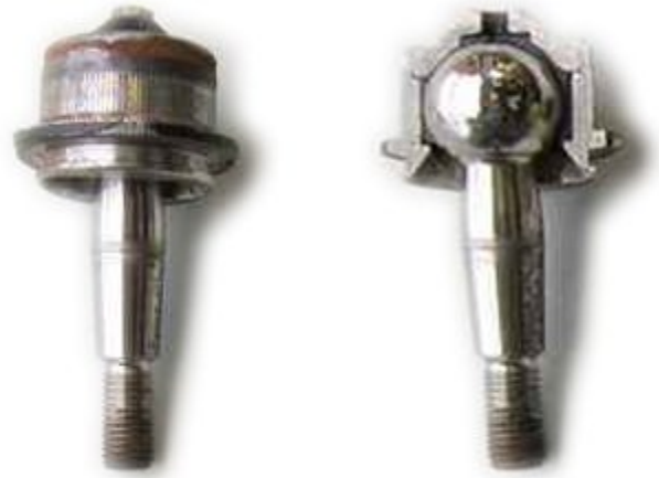
A typical ball joint with cutaway view
